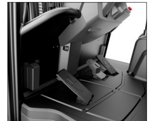
Dual pedal system - forward and reverse.
